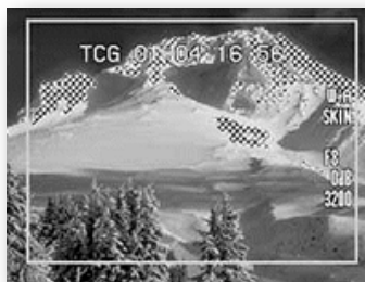
At a setting of 100 IRE the zebra stripes show the mountain peaks to be over exposed and will lose all detail.
