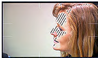
At a setting of 80 IRE the zebra stripes indicate a correct skin exposure for this woman
