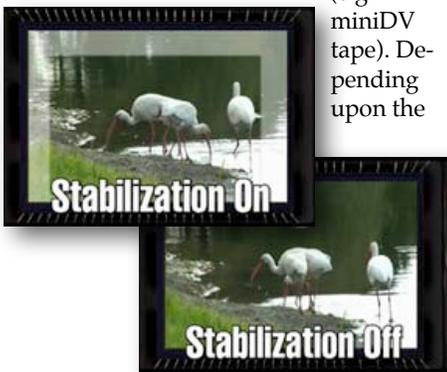
image sensor's size and the amount of correction required, EIS can reduce the effective resolution by as much as 40%. In most cases the loss of resolution is not that high, and so EIS is usually beneficial when shooting hand-held.
