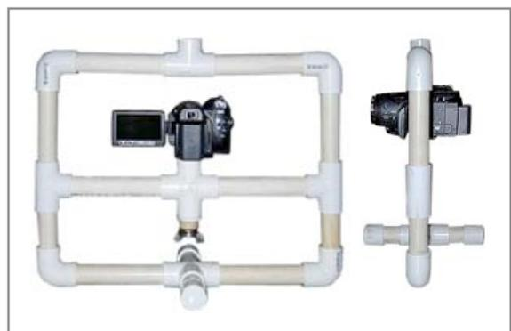
sag in the top piece may be due to the fact that my PVC pipe cutter does not cut a true 90 degree edge, not that the sag affects the stiffness.
